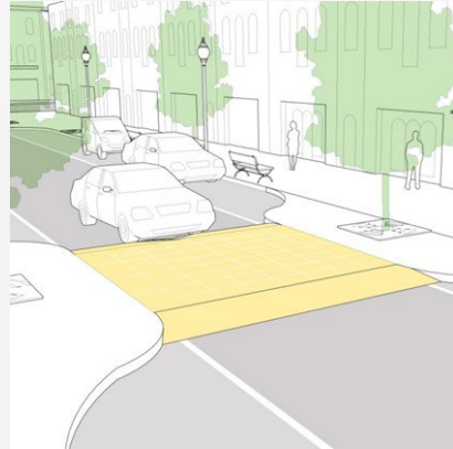
Speed table / Raised Crossing
