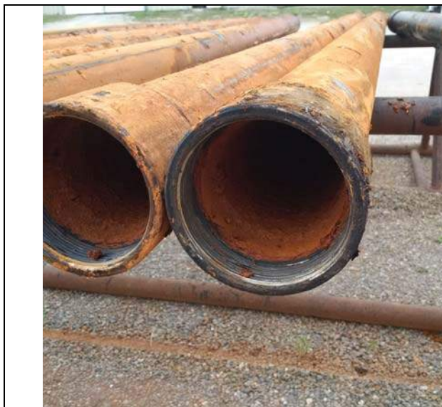
100mm drop pipe prior to cleaning
