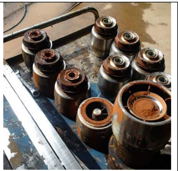
Pump dissembled and ready for cleaning
