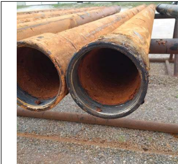
100mm drop pipe prior to cleaning
