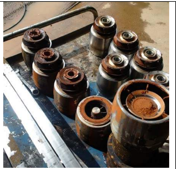
Pump dissembled and ready for cleaning
